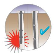
AQUAPLUS OROFLEX WELL CAN EASILY BE INSTALLED IN IRREGULAR WELLS. Aquaplus Oroflex Well can be installed with centering devices, and technical problems can thus be avoided.
